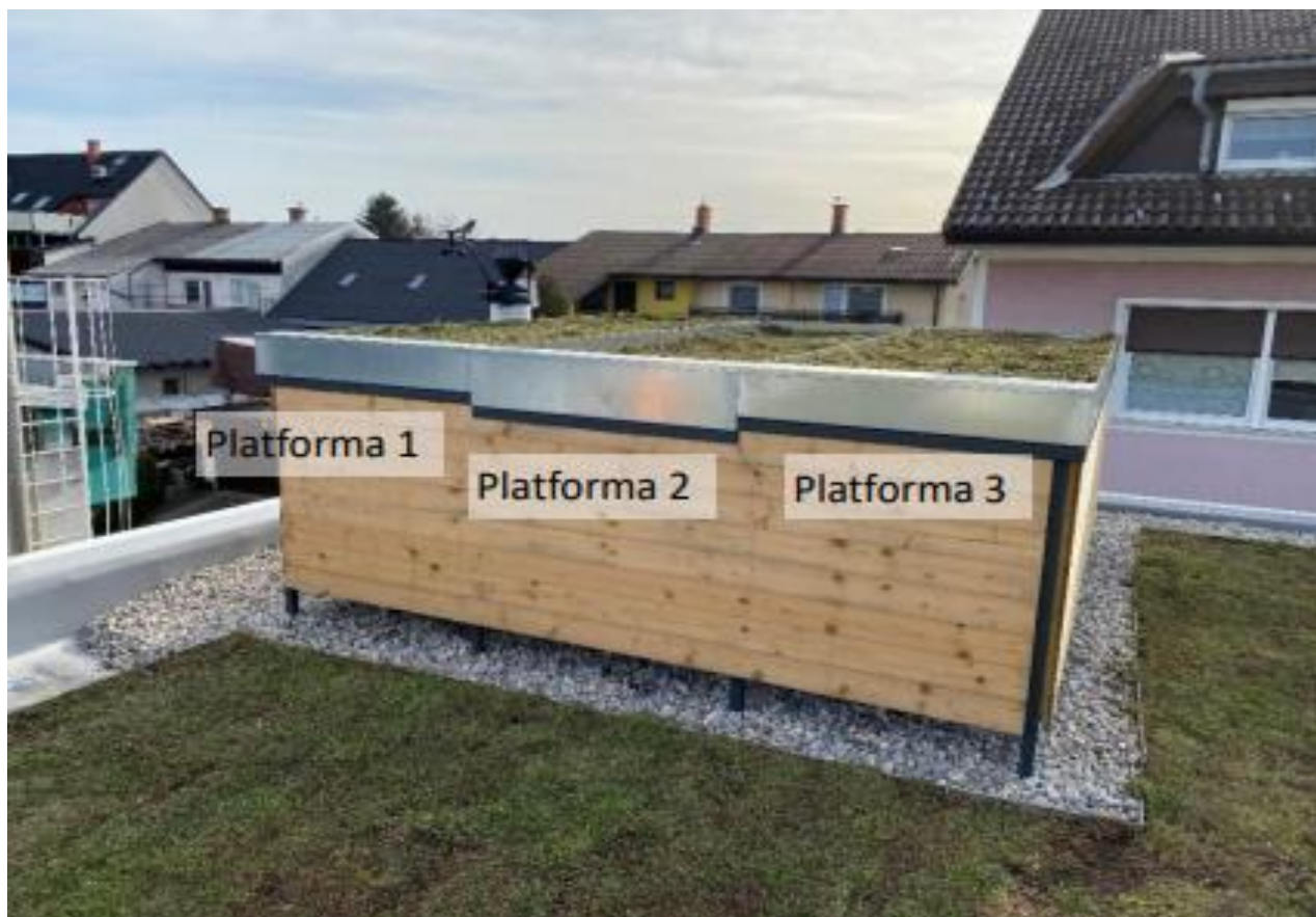
Photo: Platforms with Green Roofs for advanced Stormwater management, located in Maribor, Slovenia (left) and Bunnik, the Netherlands (right).
