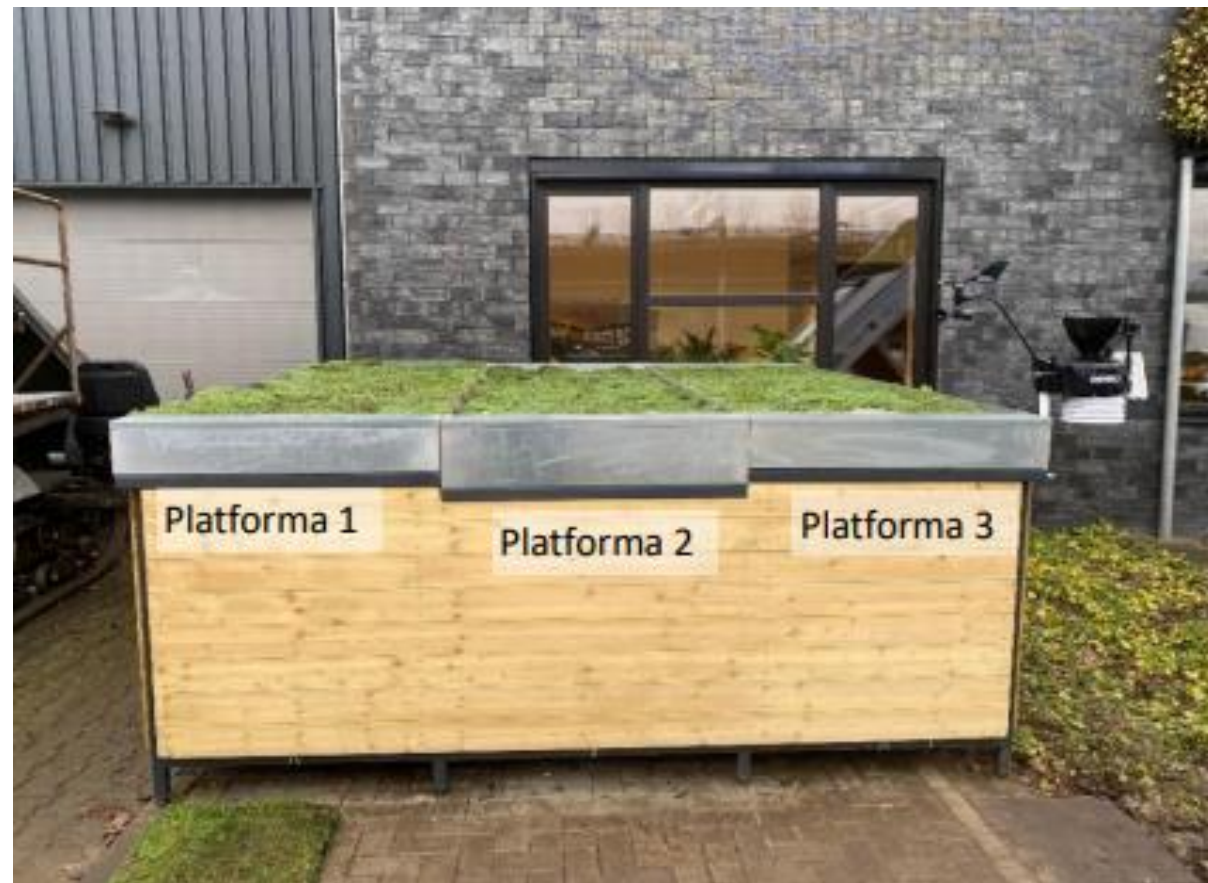
Photo: Platforms with Green Roofs for advanced Stormwater management, located in Maribor, Slovenia (left) and Bunnik, the Netherlands (right).
