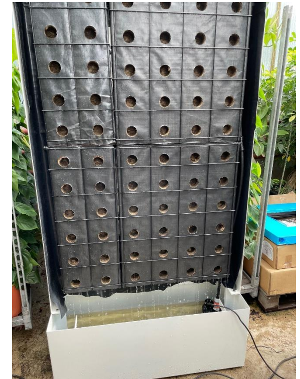
Wallflore-Prototyp (Cloudgarden/Ruof): Rockwool covered with perforated HDPE film
